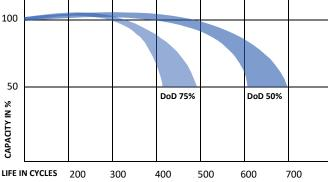
\* Cycle life is measured with a discharge current 0,2C, charged 16h and rest capacity of 2/3 Cn
